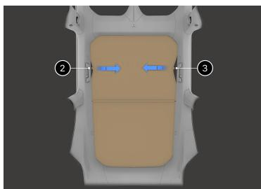
8. Ensure the flat surface of all rear sunshade clips is securely between the trim and the glass.
